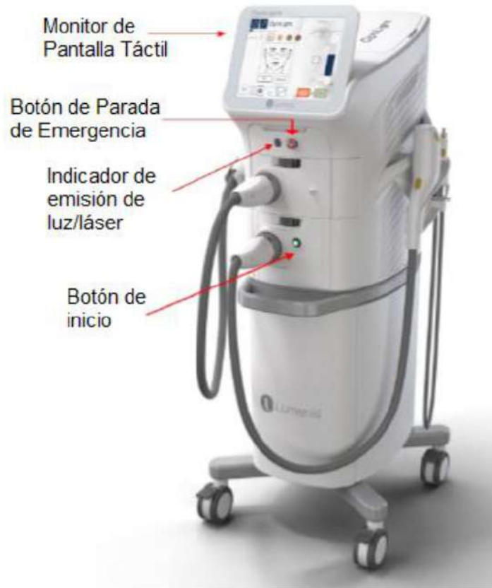
Figura 9.1: Panel de Control Principal
